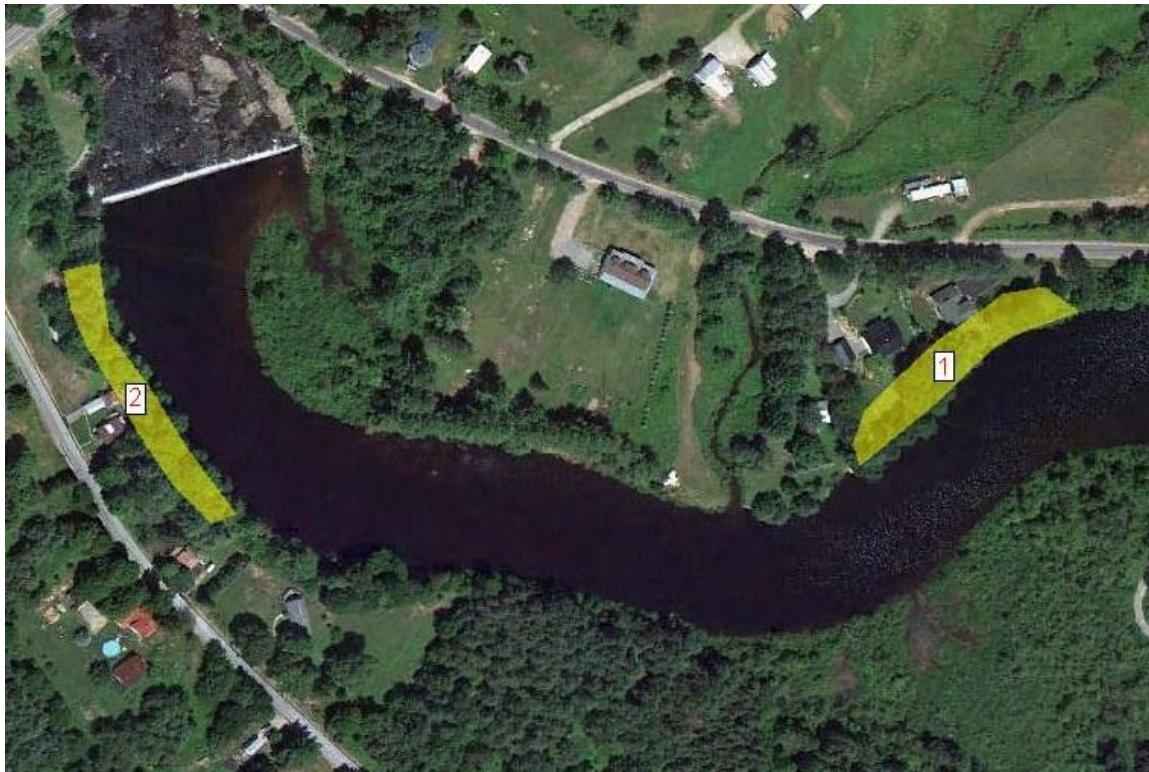
FIGURE 3-2. AREAS OF CONCERN FOR BANK INSTABILITY AFTER THE HAWKINSVILLE DAM IS REMOVED
